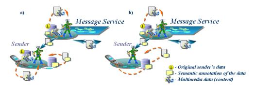
FIGURE 70 Sender's original data transmission: (a) Duplication and (b) Shifting the data to the service side
