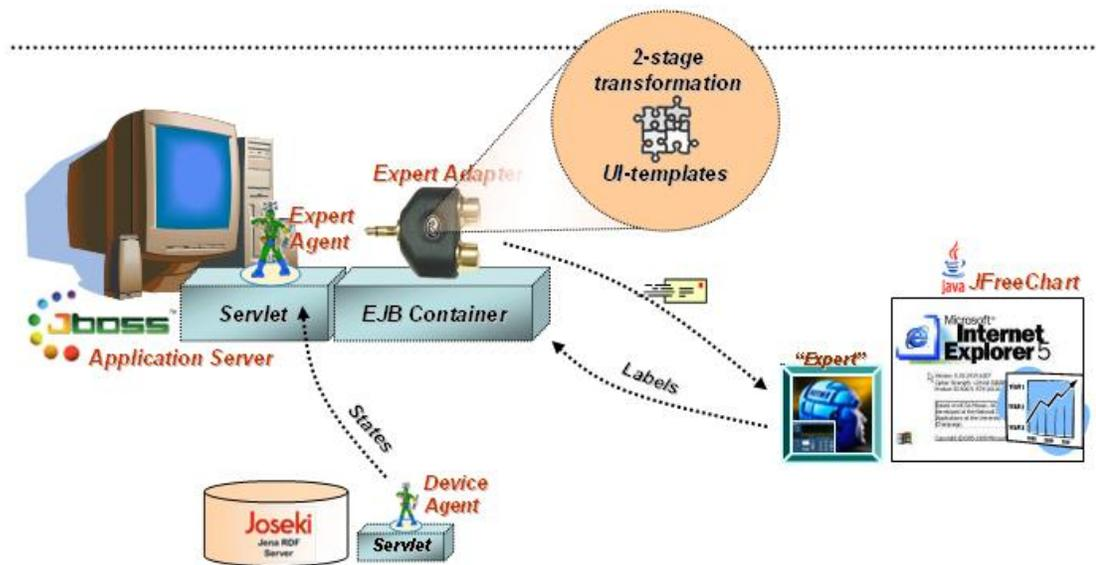
**Figure 41** - Implementation architecture of the human expert adapter
