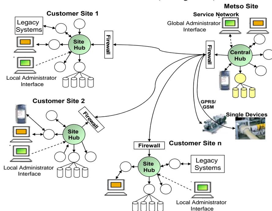
**Figure 50** – Metso SiteHub network architecture
