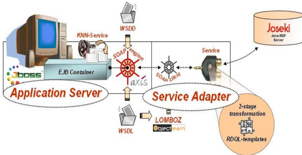
**Figure 40** - Implementation architecture of the Web Service adapter
