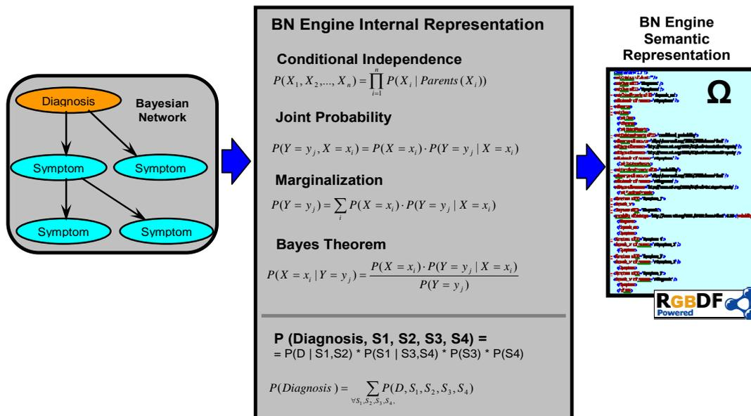
Figure 20 - Sample of a Bayesian Network reasoning engine internal and semantic representation
