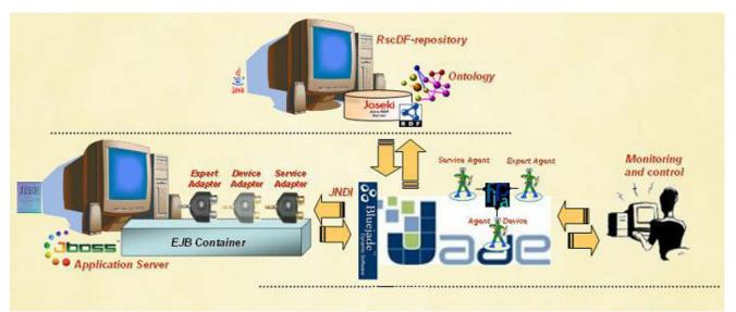
Figure 45 - Architecture of the SmartResource prototype environment, v. 2.0
