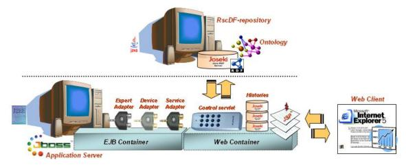
Figure 39 - Architecture of the SmartResource prototype environment, v. 1.0
