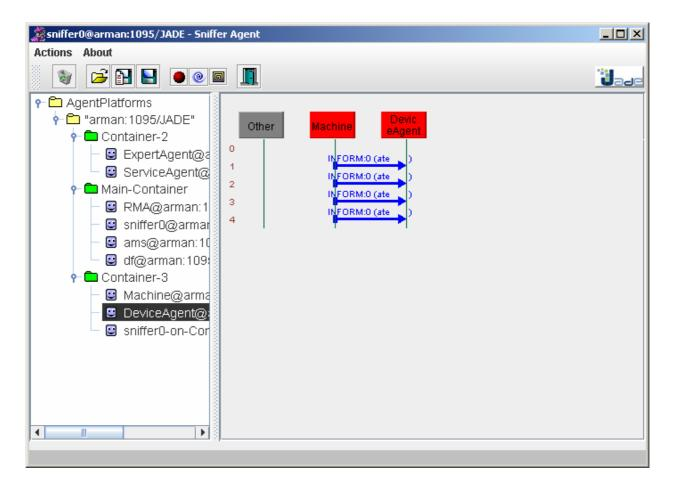
Figure 7 - Message flow from AgentDeviceGenerator to DeviceAgent
